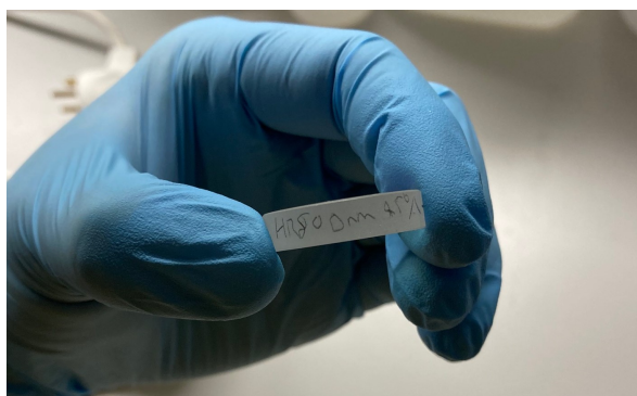
Figure 6.21: A labelled mirror showing clearly the design wavelength, designed angle of incidence, and coated side.
